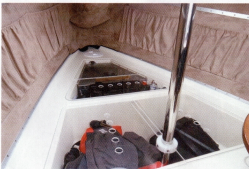
Bunk tops are clear acrylic. The water tank is in the bow, together with the battery, water pump and battery charger.
